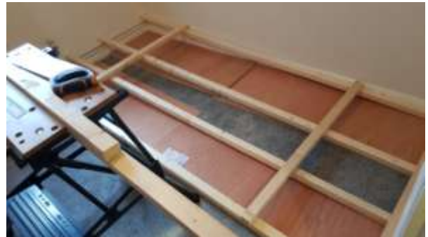
A solid foundation: the beginnings of an N-gauge model railway, with 56 half-mortice joints to cut by hand
